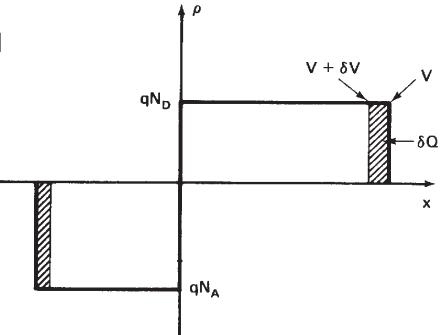
So far, we considered the p-n junction in equilibrium (i.e. no net currents). However, if an external bias  $V_a$  is applied, the system is not any longer in equilibrium, but steady state (i.e. charge density does not change w. time).
