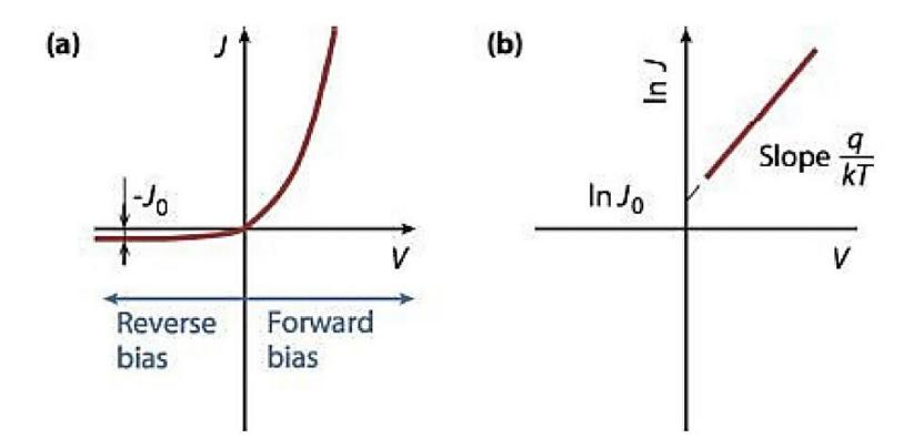
J-V characteristic of a p-n junction; (a) linear plot; and (b) semi-logarithmic plot.
