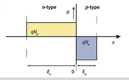
In the *abrupt junction approximation*, the <u>electric field</u> and the <u>potential</u> can be calculated simply with Poisson's equation:  $\frac{d^2 \psi}{dx^2} = -\frac{d}{dx} = -\frac{\rho}{\epsilon_0 \epsilon_m}$
