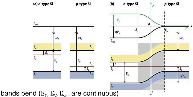
$\Rightarrow$  Internal E-field is determined by a so called *built-in-voltage*
